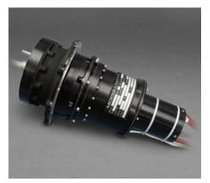
The single axis Type 2 Solar Array Drive Assembly (SADA) is based on the Type 2 Rotary Incremental Actuator. The standard actuator has varied over many applications to meet mission requirements. Generally, the items that tend to vary are interface parameters and power transfer requirements. All of the represented Type 2 SADA designs are configured with harmonic drive gear sets,
